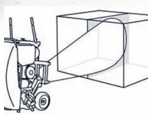
*Vertical position - Wire sawing with saw in vertical position.*
