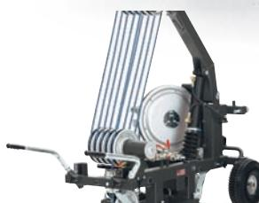
*Turning mechanism - The casters follow the direction of the wire automatically thanks to the ball bearing turning mechanism.*
