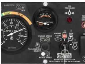
*Tachometer/bladeshaft rpm gauge - The tachometer/ bladeshaft rpm gauge on the FS 6600 D and FS 4800 D indicates engine rpm or bladeshaft rpm. Bladeshaft rpm range is colour coded to gear selection position.*
