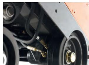
*Hydrostatic drive system - Innovative hydrostatic drive system with balanced dual motor drive system. No belts, chains or gears to adjust.*
