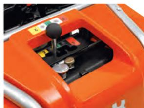
*Three speeds - On the FS 6600 D and FS 4800 D, the gearbox shift lever is used to change the output speed of the engine gearbox. Three speeds and two neutral positions are standard. The gearbox shift lever positions are colour-coded to match the blade diameter and the bladeshaft rpm decal located on the control panel. Gearbox detent locks the gearbox shift*
