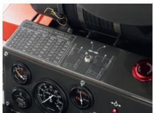
*Electric tracking system - Patent pending electric tracking system lets operator make tracking adjustments while cutting.*
