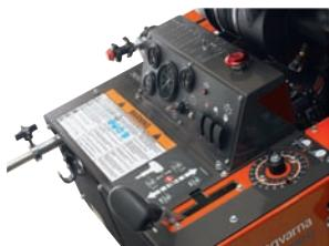
*Control panel - Control panel with temperature gauge, ammeter, tachometer and blade clutch switch.*
