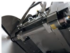
*IntelliSeal - The patented IntelliSeal blade spindle has four sealed radial bearings for strength and durability. Allows for a minimum of 500 hour maintenance intervals and a 1000 hour limited warranty.*
