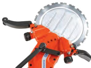
*Cutting depth - With the peripheral drive, the cutting depth is not limited by a blade spindle, and you can cut far deeper than with a traditional cutter with a centre-driven blade. The cutting depth of 260 mm (10") is sufficient to cut through a normal wall from one side.*
