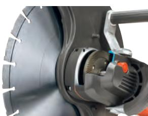
*Quick acting locks - Quick acting locks for the spindle and a large outlet in the blade guard simplifies blade replacement.*
